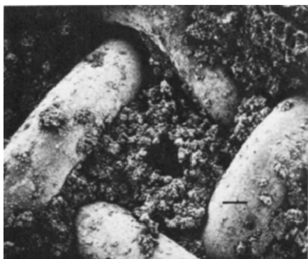
Fig. 1. A general view of the Zn(THF) electrode structure lying within a grid square of the copper gauze current collector (bar = 100 \mu\text{m} ).
